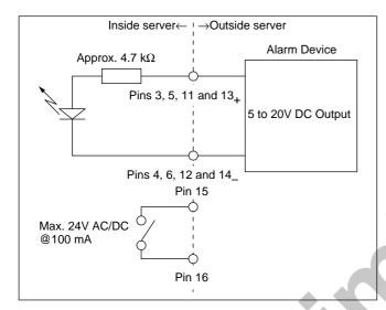
If an alarm device has mechanically switched or opencollector outputs that do not need to be electrically isolated, connect as follows.
